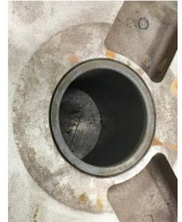
**Solution:** Pump was rebuilt using GM110.3, GRAPHALLOY Bushings with a shaft to bushing clearance of 0.006 – 0.007”. The tighter clearances were possible due to the non-galling properties of GRAPHALLOY.
