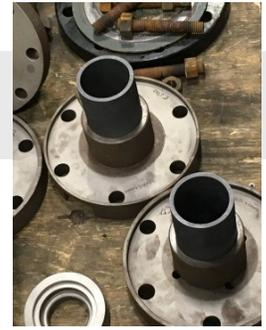
**Problem:** Pumps were fitted with nickel-chromium (Ni-Cr) bearings to handle the high temperature environment. To avoid seizing and galling, the line shaft and volute bearings were fit with 0.020 – 0.025” running clearance. However, the pumps were experiencing high vibration, approaching 1.0 inches/second peak. When the pump was disassembled, the bearing clearances had opened up to 0.030 – 0.034”.
