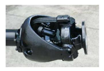
This TCVJ8C10 was used to power a luxury yacht, allowing the marine architect a choice of engine positions.
