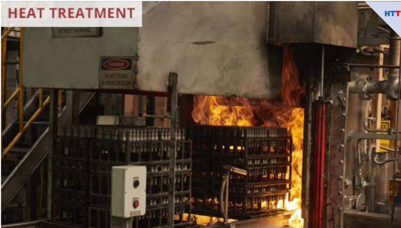
The conveyor transporting the parts has bearings to support the load and convey the product through the furnace. (photo source: Graphite Metallizing Corp)
