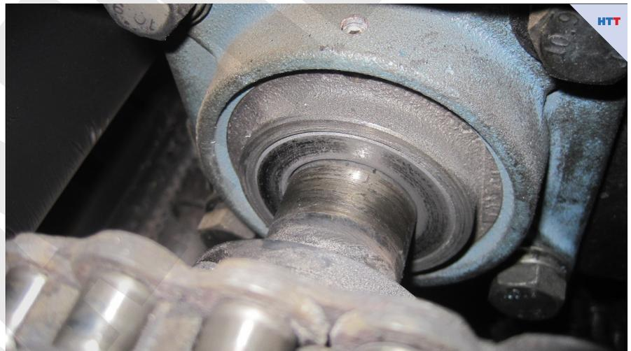
Graphalloy 4-bolt flange block in service. (photo source: Graphite Metallizing Corp)
